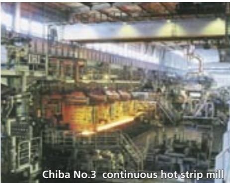
"Endless rolling" at Chiba No. 3 continuous hot strip mill
